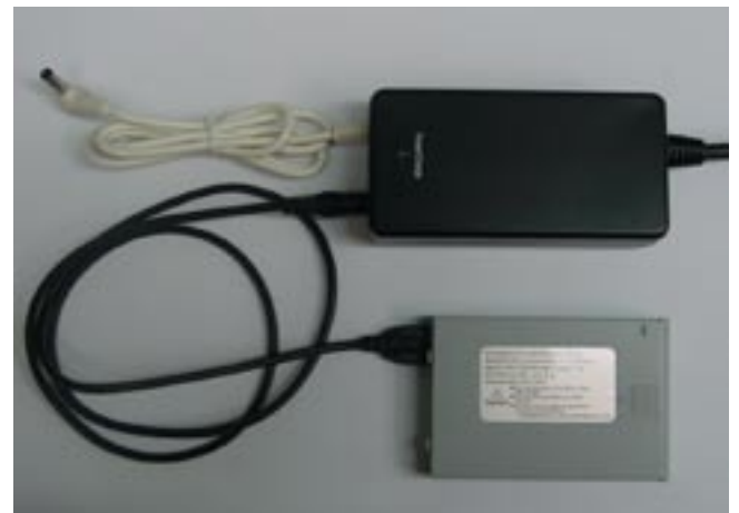
FIGURE 2-10. MPUS 300 CHARGING THROUGH AUTO-CHARGER
