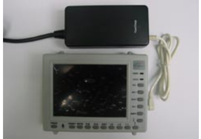
FIGURE 2-8. MPUS 300 CHARGING ADAPTOR CABLE
